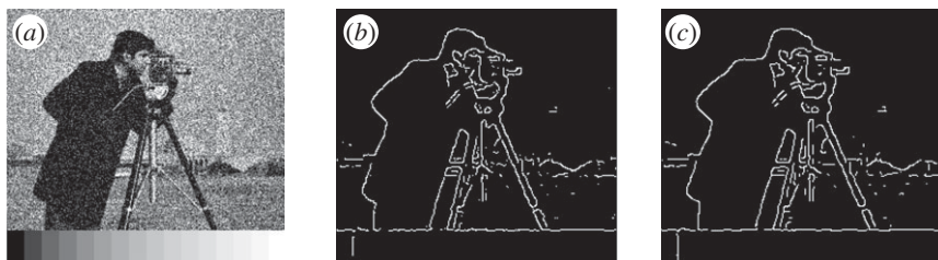
Figure 9. Comparison of edge detection performance in a noisy environment. (a) Original noisy image of Cameraman ( 256 \times 256 ), (b) Bessel integral filter ( \epsilon = 3.4 ) and (c) Jacob–Unser edge 1 filter (filter size = 13 \times 13 ).
