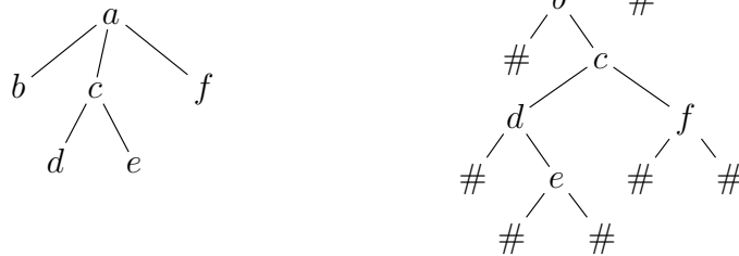
Figure 24: The tree a(b, c(d, e), f) and its firstchild-nextsibling encoding a(b(\#, c(d(\#, e(\#, \#))), f(\#, \#))), \#) .
