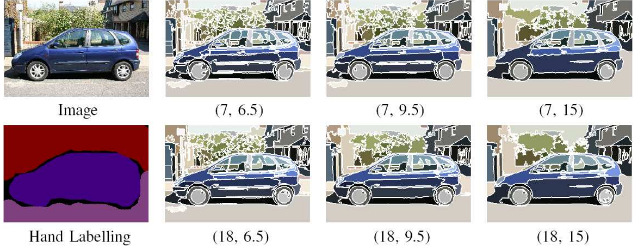
Fig. 5. Generating multiple segmentations. The figure shows the segmentations obtained by using different parameters in the mean-shift algorithm. The parameters used for generating the segmentation are written below it in the format (h_s, h_r) , where h_s and h_r are the bandwidth parameters for the spatial and range (colour) domains.
