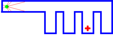
Fig. 1. The robot starts from the extreme left position, heading to the right; its target location is indicated with a cross.
