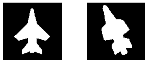
Fig. 1. Left: Contours \mathcal{C}_1 and \mathcal{C}_2 with 6 corresponding points p^{(i)} \leftrightarrow q^{(i)} . Right: optimal alignment of \mathcal{C}_2 to \mathcal{C}_1 and \mathcal{C}_1 to \mathcal{C}_2 .
