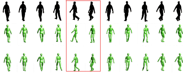
Fig. 2. Every 20th frame from a circular walk sequence, Top Row: Input Silhouette, Middle Row: Model Pose Estimate, Bottom Row: Ground Truth. The box indicates bad estimates by our model
