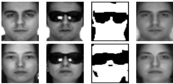
Figure 6. Results on partially occluded faces. Left to right: gallery image, probe image, visibility estimation and reconstruction ( \lambda = 50 ). The outlier histogram was re-estimated at each M-step.
