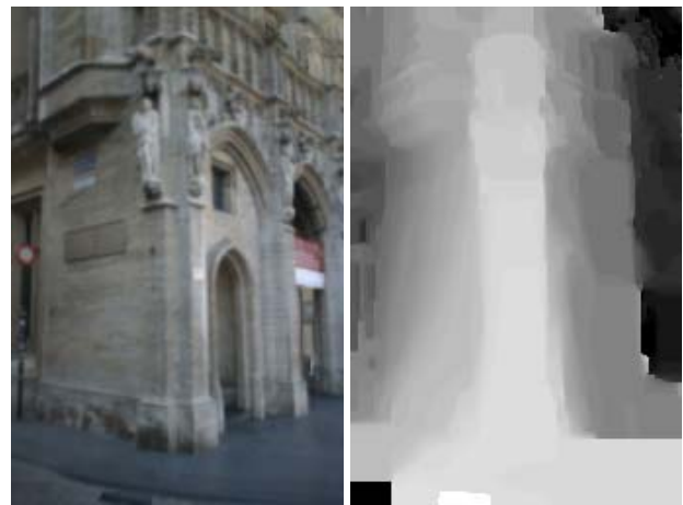
Figure 4. Ideal image y^* and depth estimate, computed from the three input images shown in fig. (3). Notice that the woman has disappeared from y^* and that a depth and colour value is assigned to these pixels by matches in the other views.
