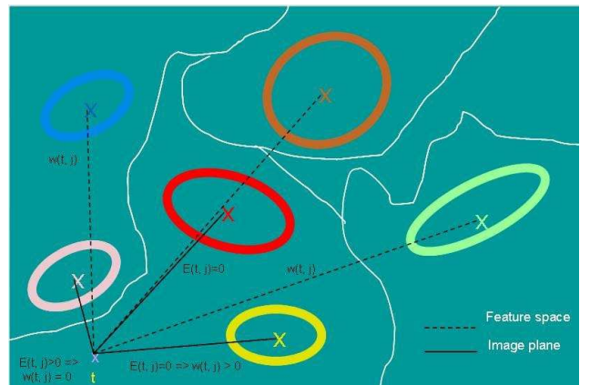
Figure 1. Combining local features and edges in the EM learning process. Edge map is overlaid in white. Gaussians in the trained model are shown as ellipses. First, the weights from point t to each Gaussian j ( w_{tj} ) are computed. For those Gaussians with high posterior probability (the three nearest ones in this example), a straight line is drawn and the function E_{tj} determines if it intersects an edge. Such is in fact the case for one of the Gaussians and the corresponding w_{tj} is set to zero. There are two remaining Gaussians for which no edge is intersected.
