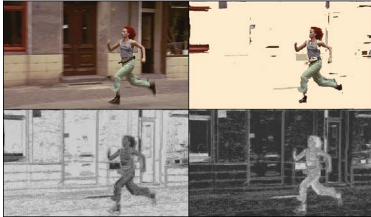
Fig. 4. Image segmentation with max-marginal probabilities. The first image is a frame of the movie Run Lola Run . The second shows the binary foreground-background segmentation where the aim was to segment out the human. The third and fourth images shows the confidence values obtained by our algorithm for assigning pixels to be foreground and background respectively. In the image, the max-marginal probability is represented in terms of decreasing intensity of the pixel. Our algorithm took 1.2 seconds for computing the max-marginal probabilities for each latent variable label assignment. The time taken to compute the MAP solution was 0.3 seconds.
