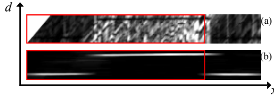
Figure 3 – DSI's slices obtained from a conventional stereo matching algorithm (a), and obtained by the growing aggregation algorithm (b)
