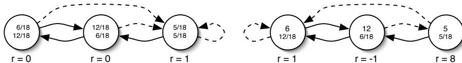
Fig. 1: Left: Baxter et al.’s simple 3-state POMDP. States are labelled with their observable features and instantaneous reward r ; arrows indicate the 80% likely transition for the first (solid) resp. second (dashed) action. Right: our modified, more difficult 3-state POMDP.
