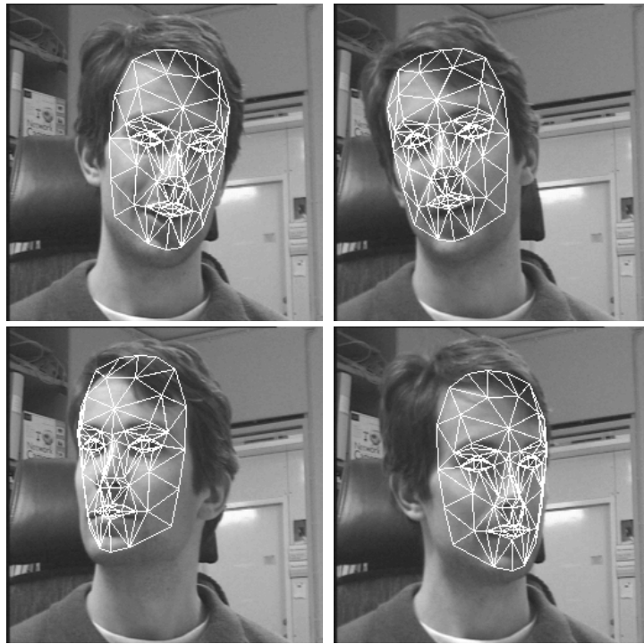
Fig. 3. Particle filter-based 3D head tracking with a statistical facial texture model.
