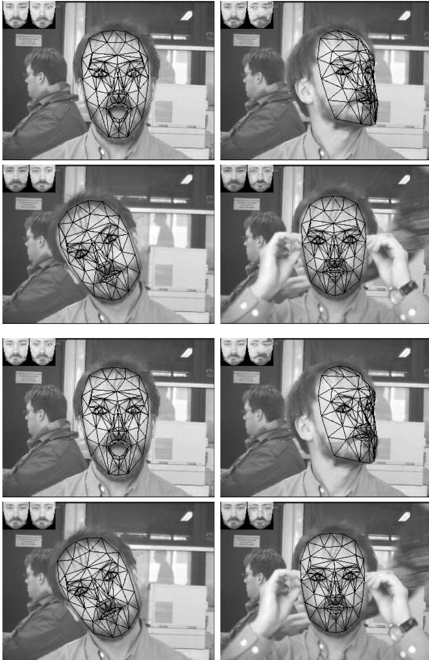
Fig. 9. Face and facial animation tracking results obtained with a 708 frame long sequence using the gradient-based registration method. At the end of the sequence the person is putting on his glasses. The two upper rows display tracking results obtained without any temporal downsampling. The two lower rows display tracking results obtained when every fourth image was used, i.e. the temporal downsampling is set to four.
