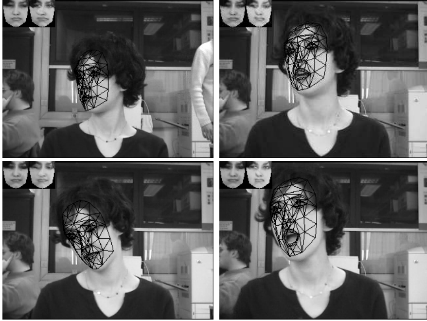
Fig. 5. Our real-time framework for tracking the 3D head pose and the facial animations with an appearance-adaptive model. The sequence length is 800 frames.
